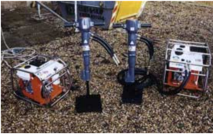
These new 'low vibration' hand held hydraulic breakers will complement Panther's existing 'semi-vibration' range.
