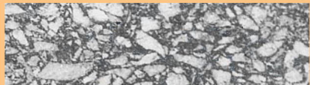
Sample 2 - The Dual Force plate compactor achieves a much lower void content. This half of the reinstatement will last 100% longer.
